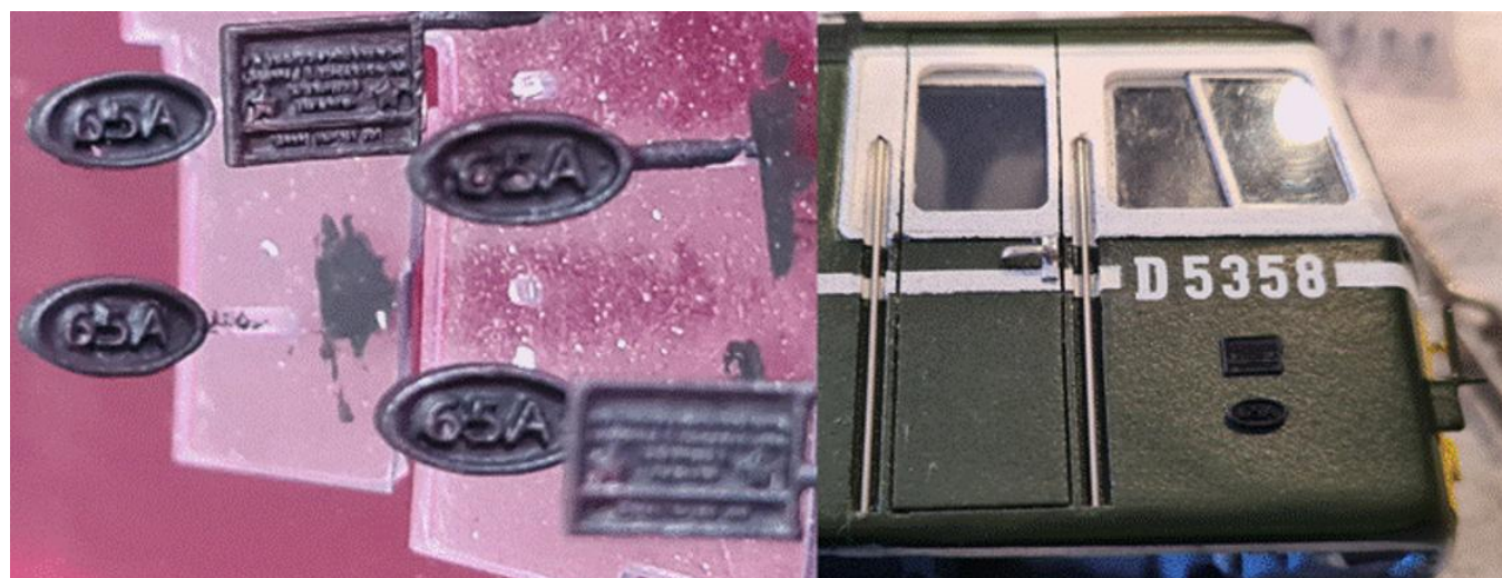
The door handles & rails and builders & shed code plates all fitted.
