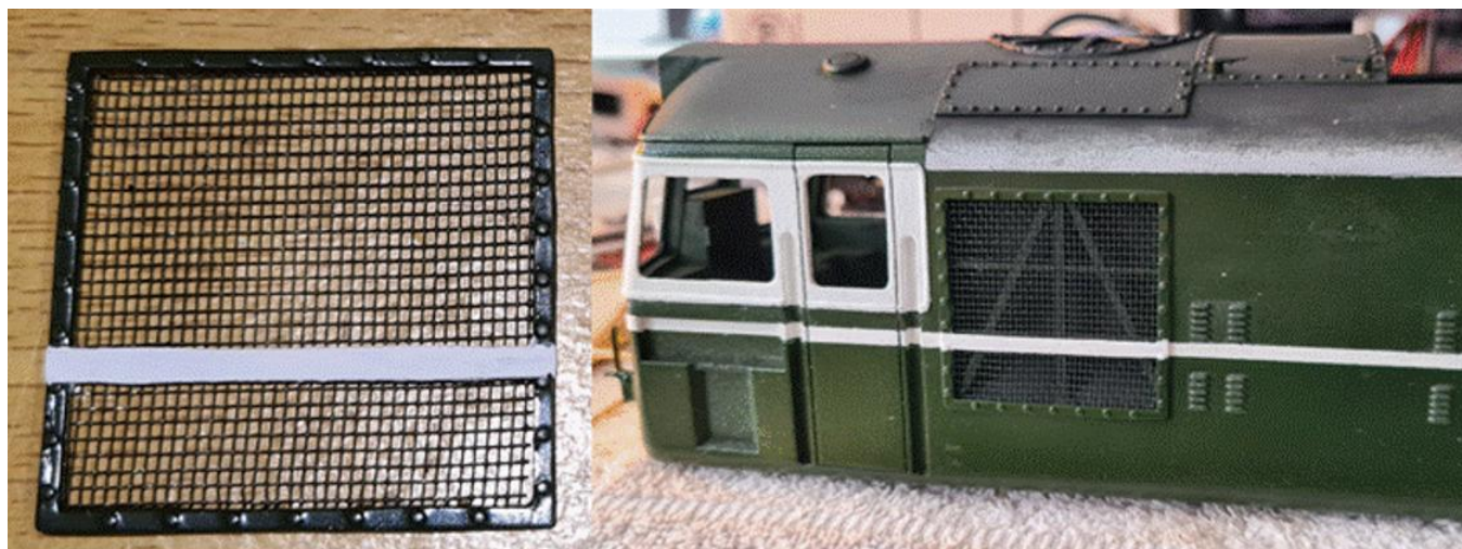
The air intake grill and frame painted and mounted.
