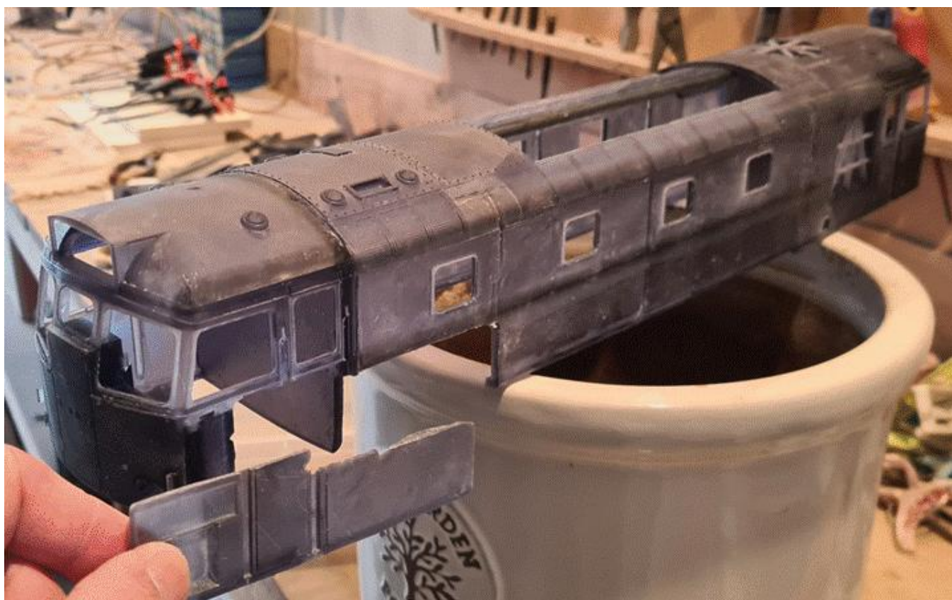
The replacement part cut from a second print, that had been angled the opposite way when being printed, being offered up to check the fit.
