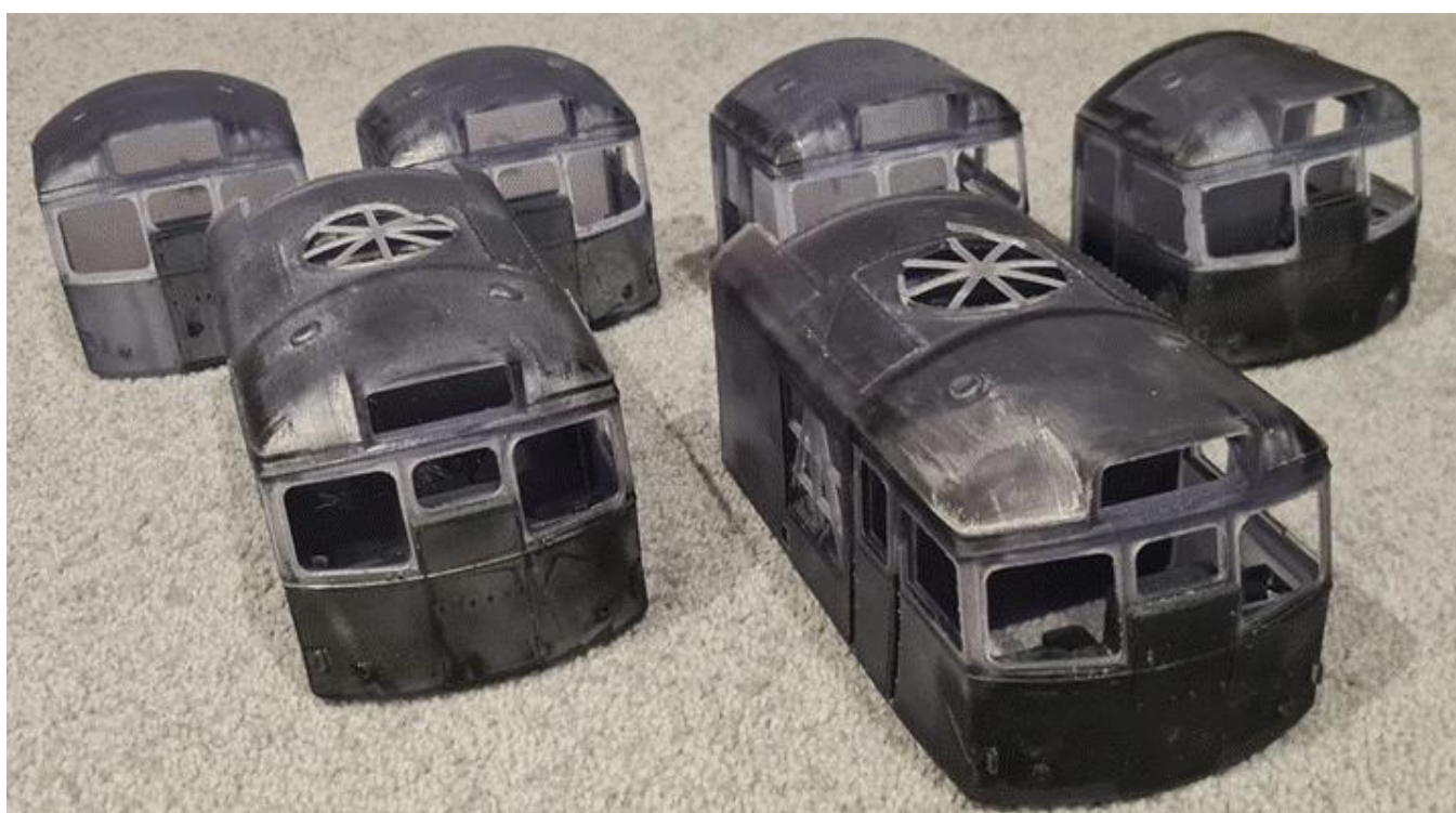
A suite of trial cab prints, each an improvement on its predecessor. There are still problems with the latest (closest) with the fan frame peeling off. This was fixed by creating a tube that passed through the roof and nestled into the frame. With 3D artwork, what appears to be a solid joint sometimes isn't!
