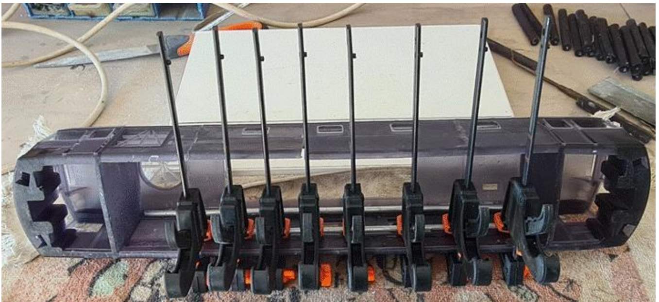
Parts being glued together with stainless steel reinforcing rods added for reinforcement and to keep the sides aligned and straight.
