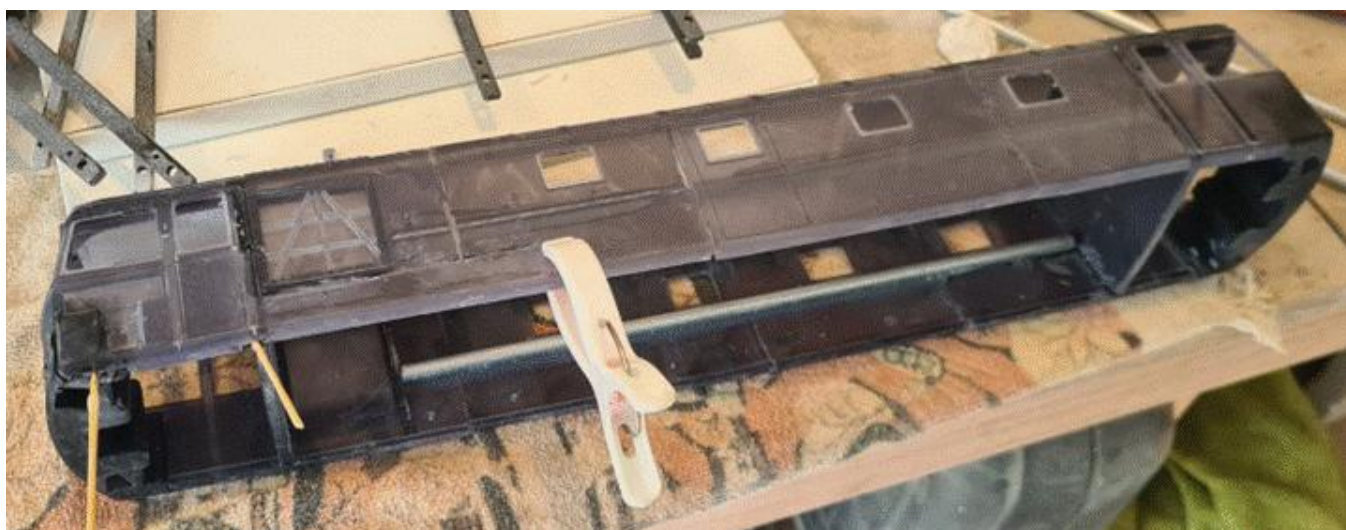
The replacement part cut from a second print, that had been angled the opposite way when being printed, being offered up to check the fit.
