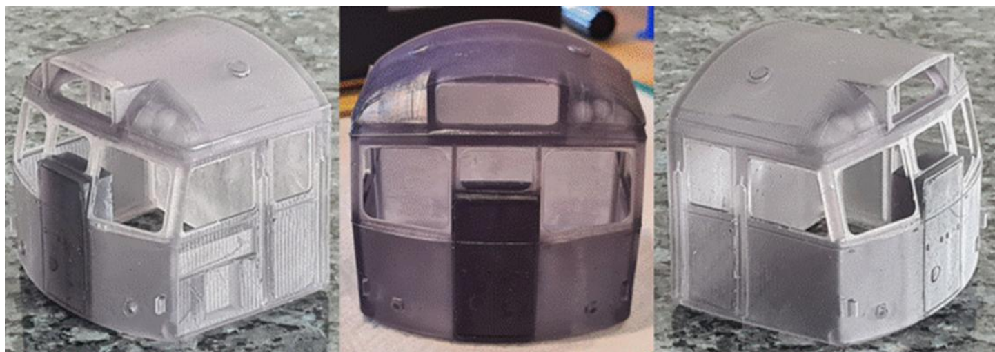
A test print of a completed cab (without the control desks at this point).
