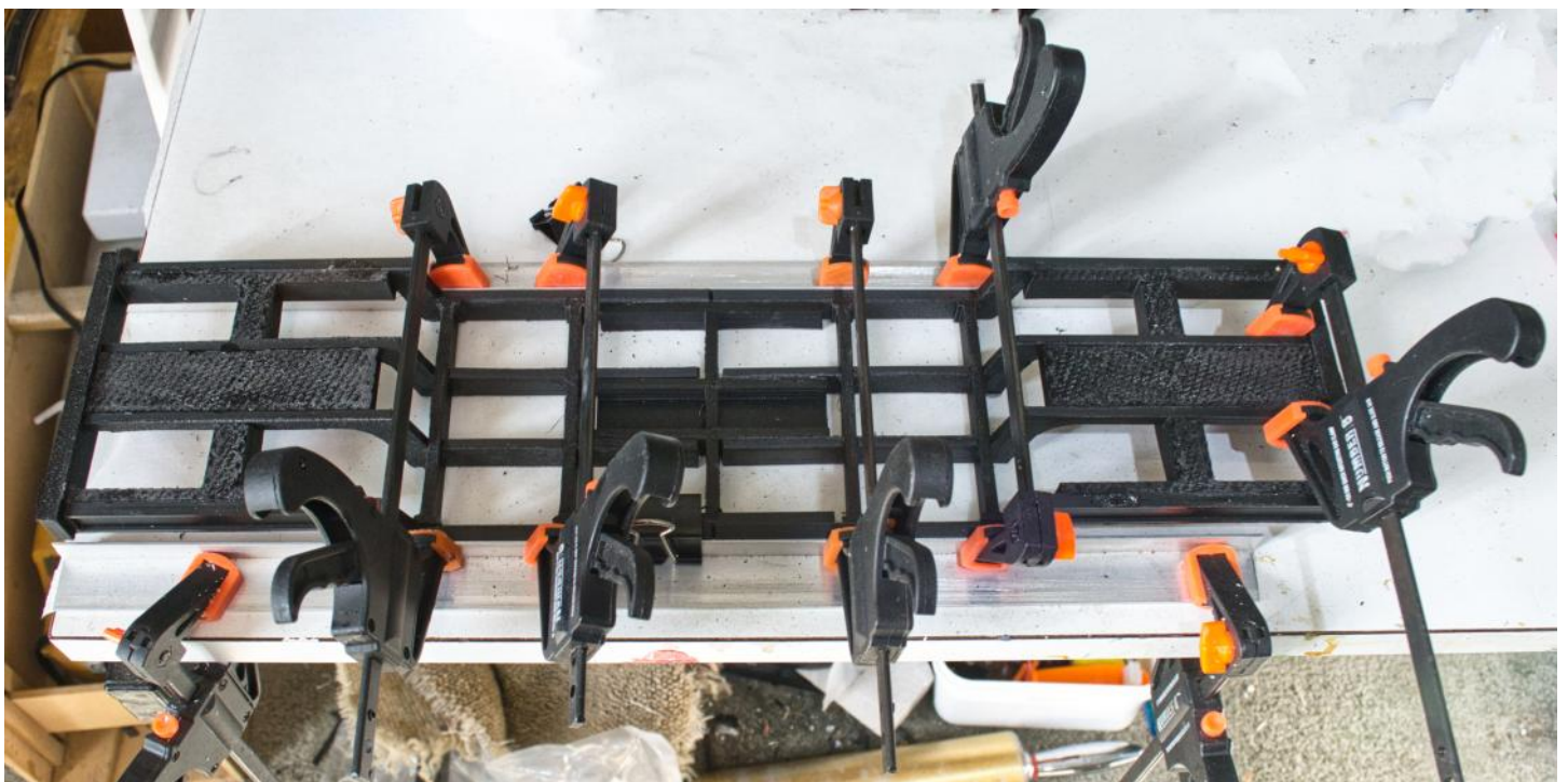
Clamping both sections together, note the right angle to keep it square.
