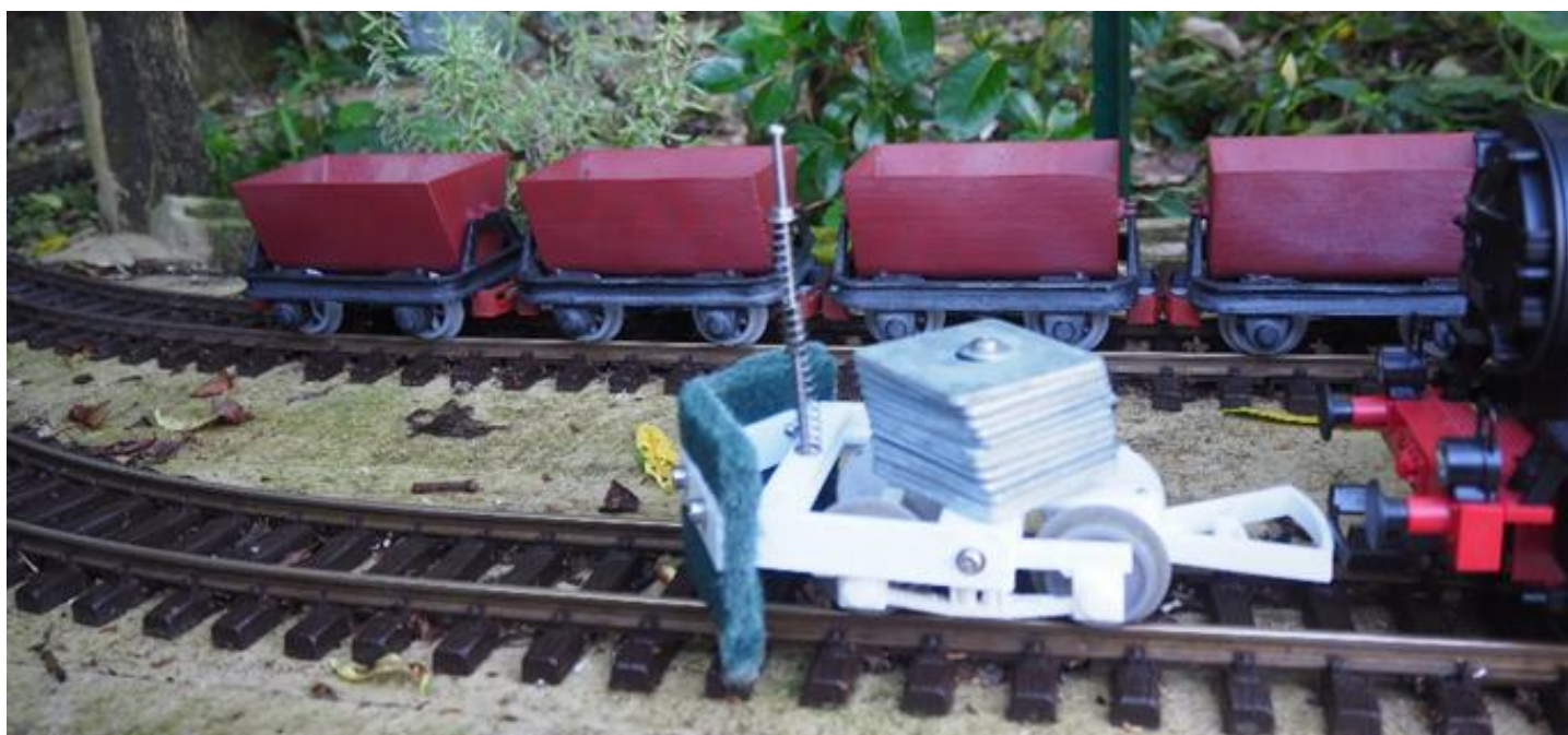
David Humble constructs his own rolling stock mostly from self-designed 3D printed parts. His scratch-built rail cleaner is in the foreground - Photo Tony Christie.
