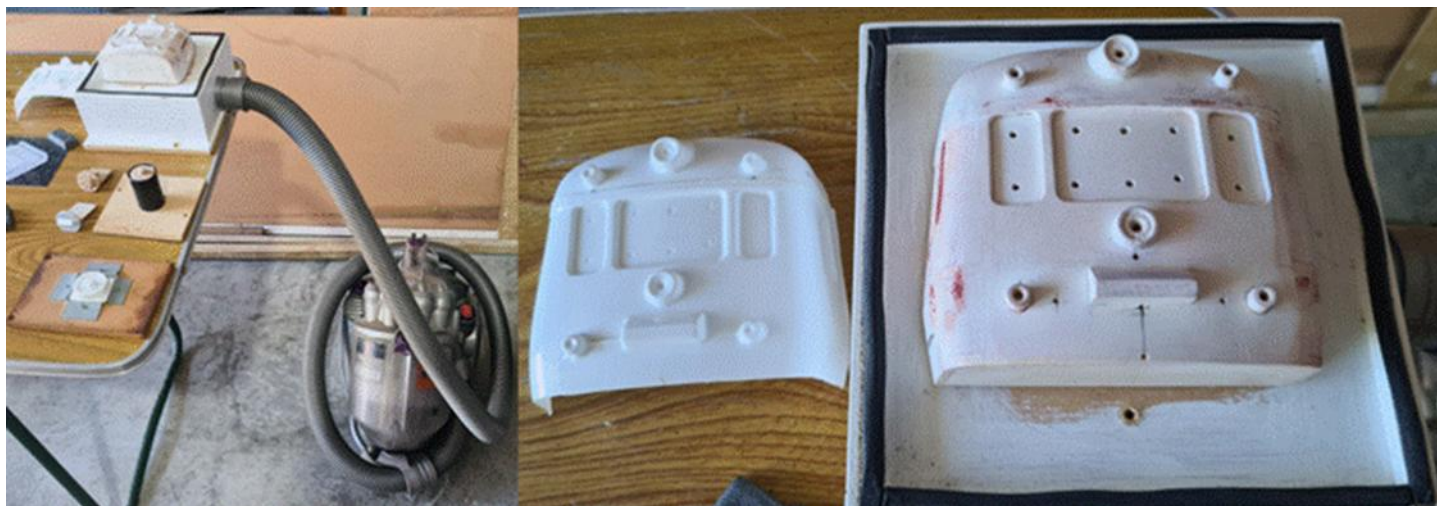
The vacuum forming system created by Dean with a pattern and resulting moulding on the right.
