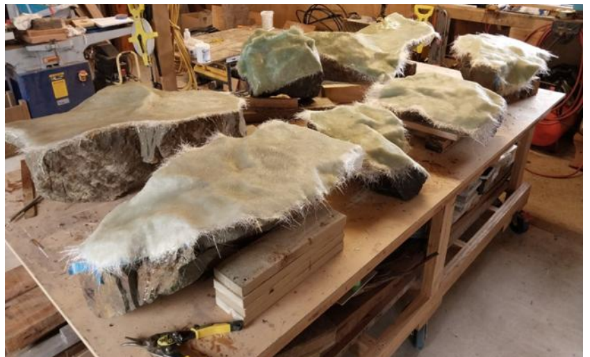
I did about 30 layers of latex, ending up with 3 -4 mm thick moulds.
