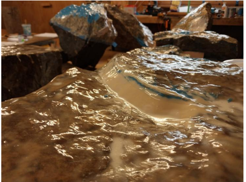
I did about 30 layers of latex, ending up with 3 -4 mm thick moulds.
