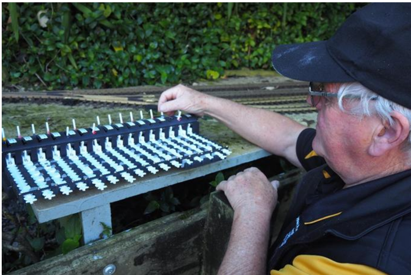
Dave Allen examining the manual interlocking frame that will eventually be installed here and linked to points and signals by wire linkages - Photo Tony Christie.
