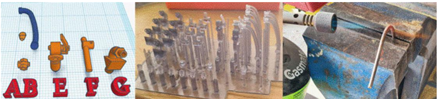
Various hose and cable fittings designed on the left, batch printed in the centre, and a section of brass tube being heated and curved to form one of the hoses on the right.
