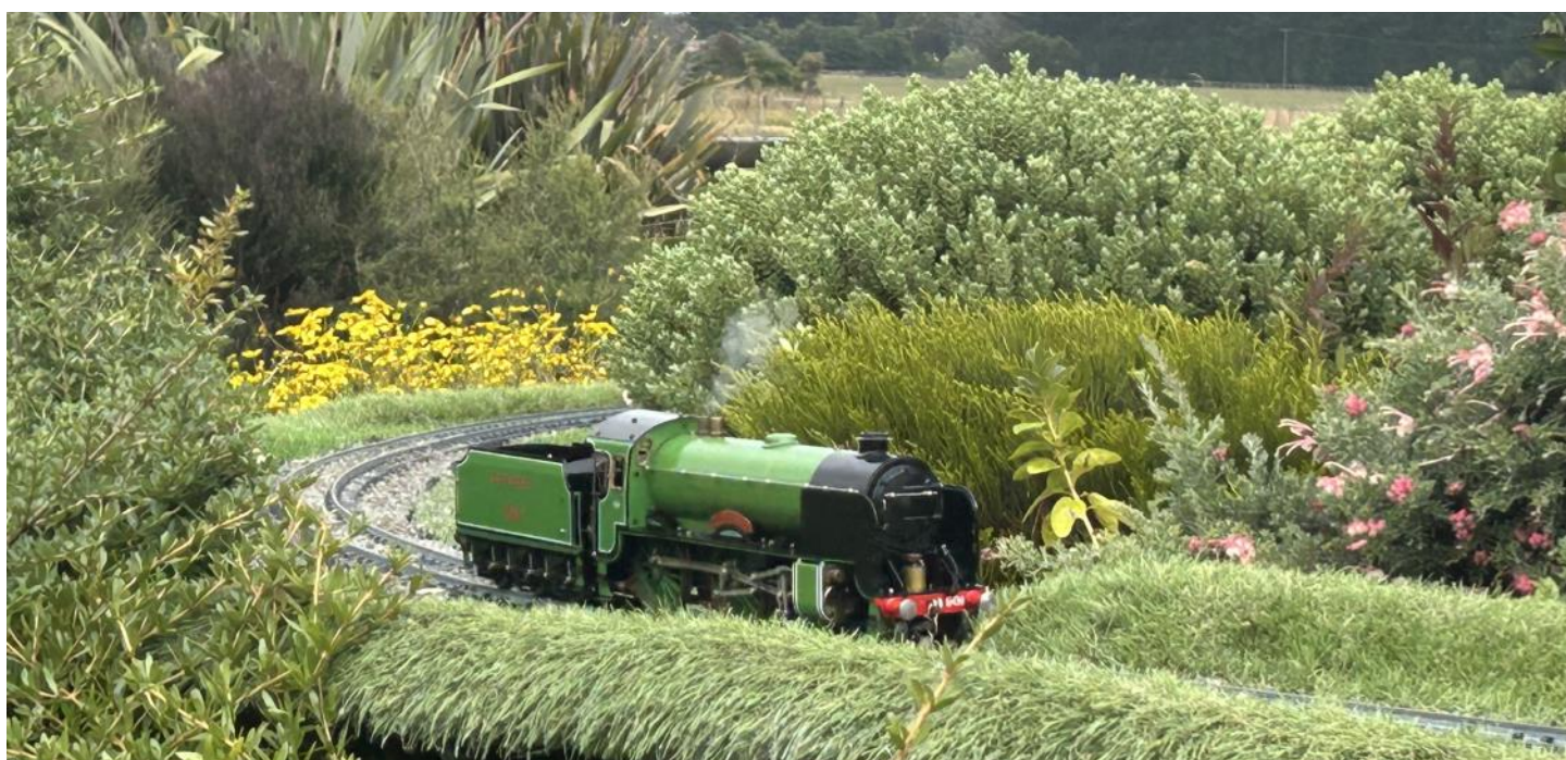
Geoff's Gauge 1 meths fired Schools negotiating the southern end of the railway as he tested out the suitability of the Te Horo Branch for the finer Gauge 1 standard of this Aster loco. With a slight adjustment to the front steps successful running ensued.
