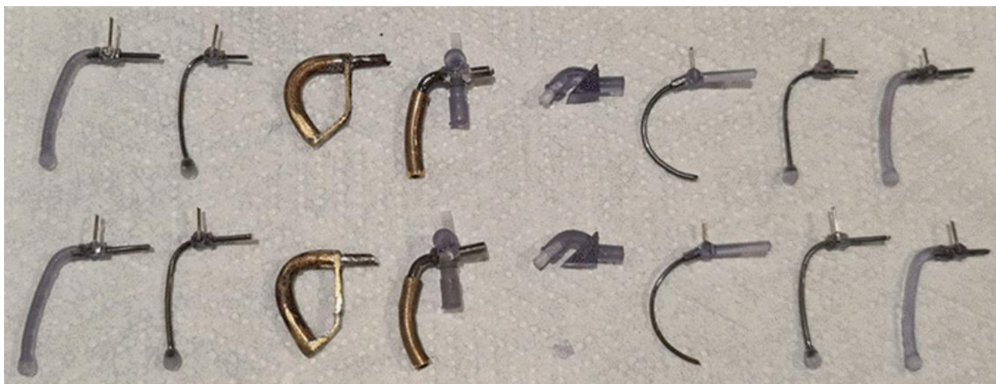
Two sets of prepared fittings for both buffer beams.
