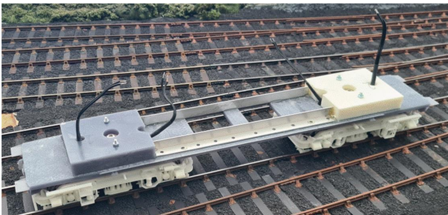
A test fit of the bogies with the underframe mounted on top to check fits. I have also drilled openings through the bolster housings to allow the passage of the wires for the four traction motors. This is one of many checks performed as design and assembly progressed. It is an important ongoing procedure on two counts. Firstly, it allows for issues to be identified earlier and thus resolved; and, equally importantly, acts as a moral booster to take pleasure in the progress being made!
