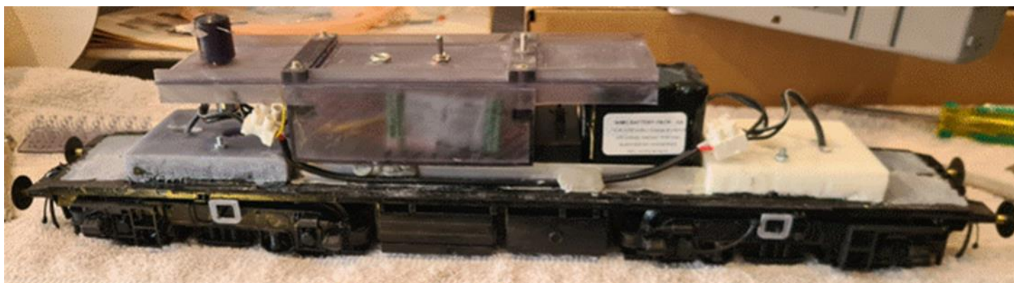
Completed chassis with electrical systems fitted in storage container with bolted on lid holding (from left to right) fan assembly, charging socket, on off switch and upended bolt for fitting and holding the locomotive body shell. N.B. the red rear light LEDs have yet to be fitted in this photo.
