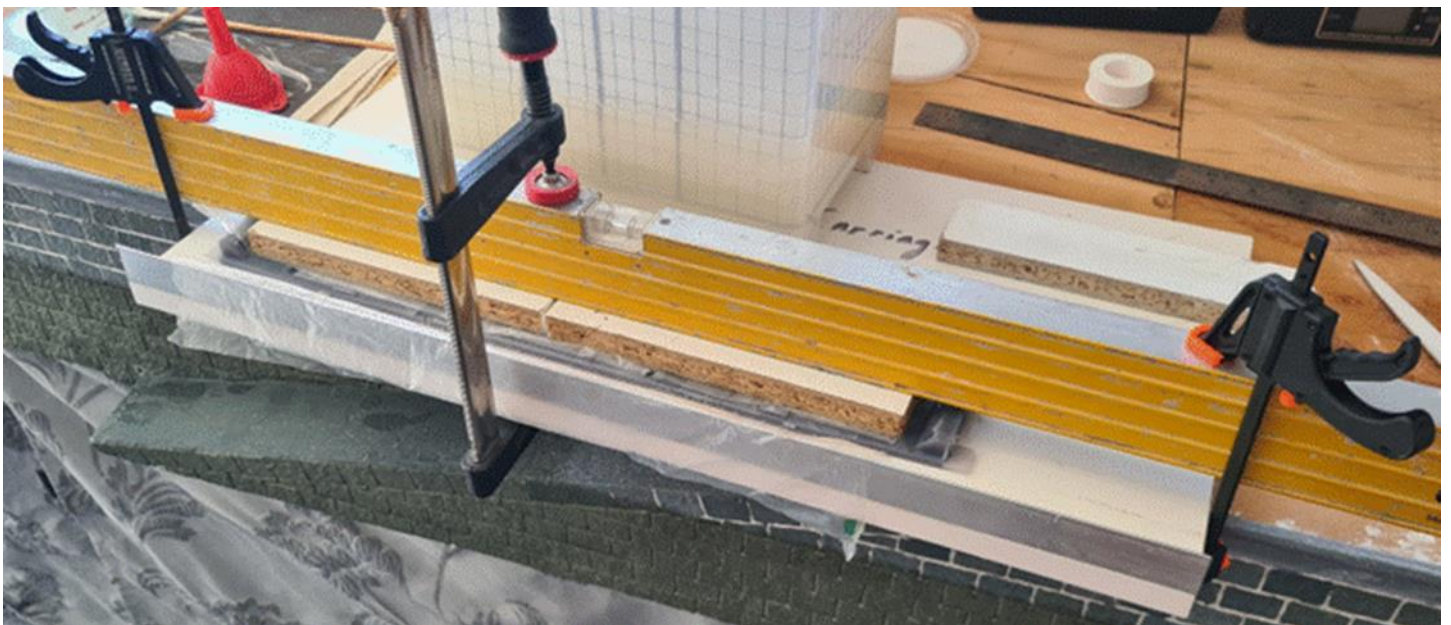
The three underframe prints cut to size and mounted in the gluing jig. This is a vital tool for this sort of work and consists of an old shelf with two aluminium angles screwed to it. The sections have been placed on a polythene film with araldite applied to each joint. They have been pushed hard against the angle lip to ensure they are true to each other. With the polythene wrapped over the top of the model, spare shelf cut offs have been placed on the top and a straight edge (spirit level) has been clamped over the whole assembly to hold it all securely in place.
