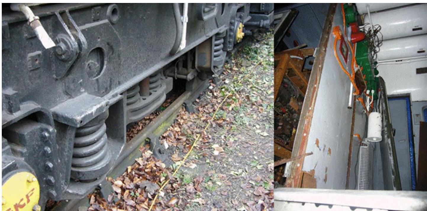
A couple of example photos taken during my survey of D5353 on the Mid Hants Railway. Having this access, allowed me to create the design with a lot more certainty than I would otherwise have had. Left, bogie frame and underslung bolster. Right, Cab interior back wall and some ceiling detail.
