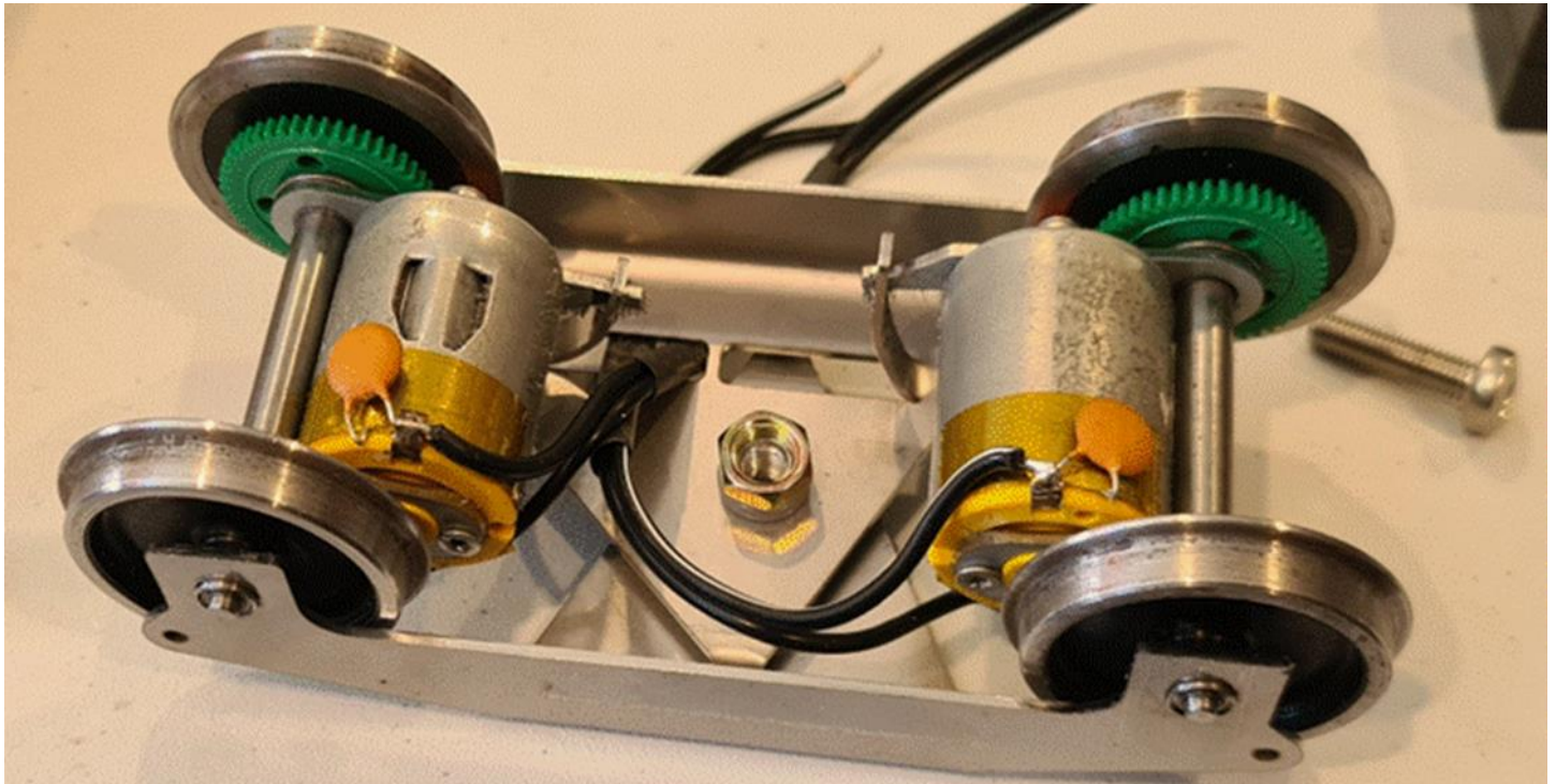
Fosworks bogie power train. These can be made to match any prototypical wheel base and diameter. The wheels were also set by Fosworks to 42mm back to backs at my request. The two sides articulate about the central pivot point. Note the roller bearings into which the axles sit.
