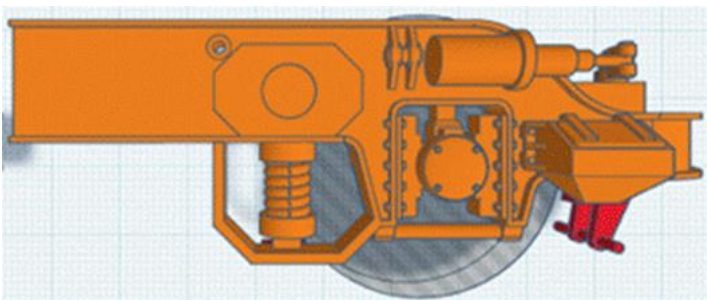
Brake cylinder, rigging and sand box added.
