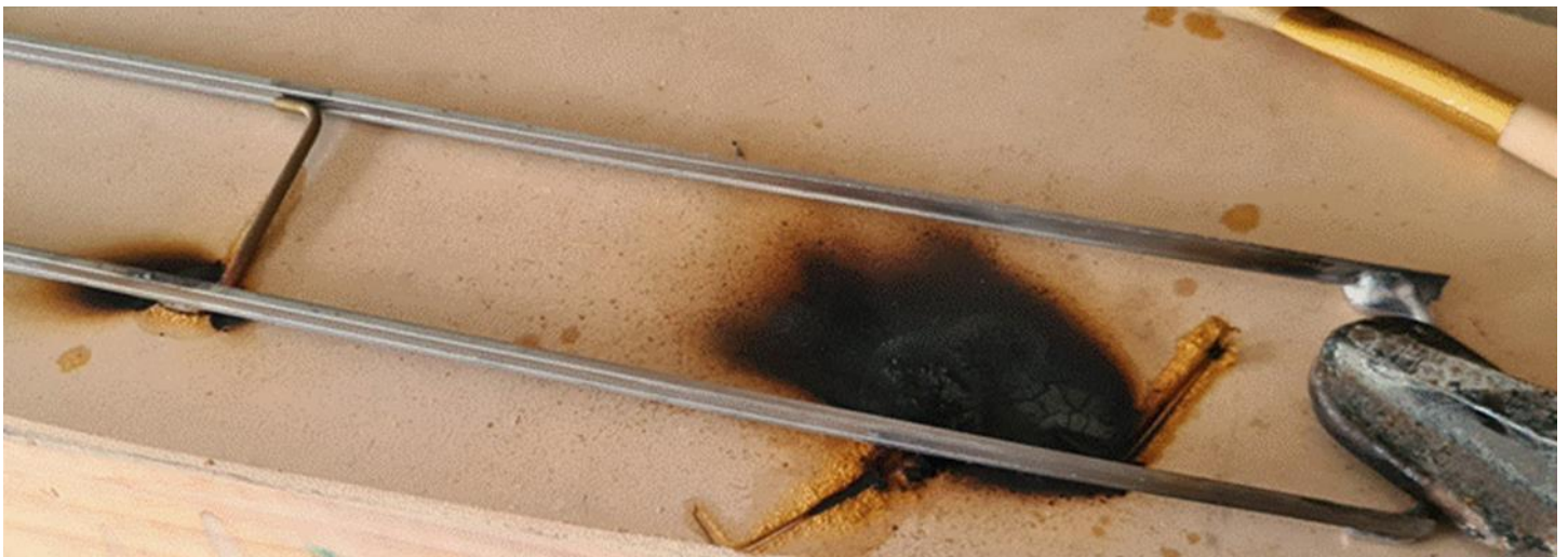
The pair of blades being soldered to a pair of tie bars
