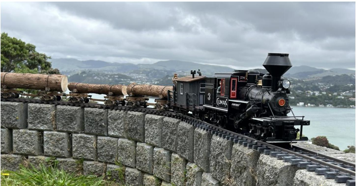
*Rodney's Climax hauled logging train. Its battery powered, the battery in the support wagon behind - Photo John Robinson.*
