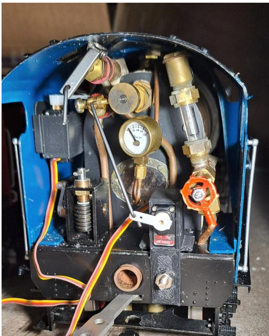
I also put in a second servo for the whistle; this A4 has a really good whistle. I had designed a bracket in Tinkercad for the steam valve servo and 3D printed this in black. For the whistle I needed a servo up higher and deeper into the cab area. I designed and 3D printed a bracket that fit into one of the window frames in the cab, this worked really well with both brackets rock solid.
