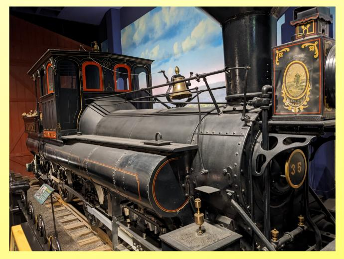
Originally 8 horses pulled one car at a time up Madison Hill. No steam engine was able to climb the 5.9% grade without slipping down the hill, as it had the steepest grade regular track in the US at that time. The Reuben Wells locomotive was built to push, not pull, trains cars up a steep hill in Madison, Indiana. The couplers holding the cars were too weak and would have decoupled if pulled. The engine was so heavy that gravity kept it on the track and prevented slippage.
