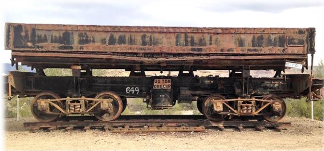
30-Ton Side Dump Ore Car in Ajo (Glenn & Janet Mitchell)
