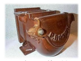
ANSWER to last month's Trivia Corner: JOURNAL BOX: The metal housing which encloses the journal (the journal bearing and wedge) of a car axle. This piece also holds the oil and lubricating deice for lubricating the journal
