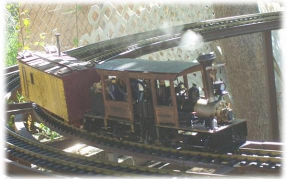
Two cylinder shay with scratch built superstructure running on inner loop
