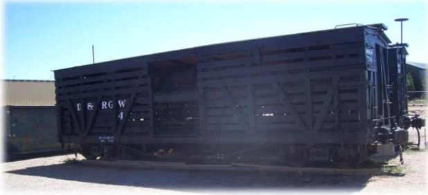
This is a nearly completed restoration of a double decked stock car (used for pigs and sheep). It lacks only some additional stenciling (such as completing the car number) and rehangng of the doors.
