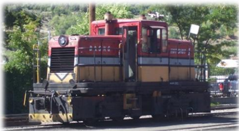
While the public trains are powered by steam the D&SNG also has seven diesels for work in the yards or on work trains. This is #1, named 'Hot Shot' a General Electric 44 ton switcher.
