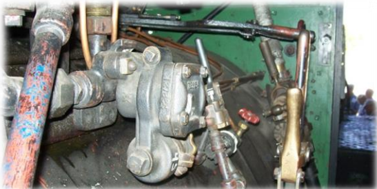
The next picture shows the engineer's side of the 315's very cramped cab. The vertical lever is the reversing gear (or Johnson bar) and the horizontal lever is the throttle.
