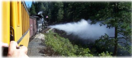
While crossing Grand Trestle the engineer took the opportunity to blow residual water out of the pistons.
