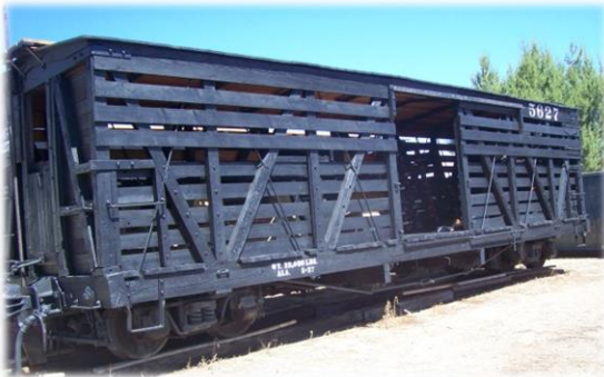
Also nearly completely restored is this single deck stock car (used for cattle) which lacks only painting and rehangng of the sliding doors.
