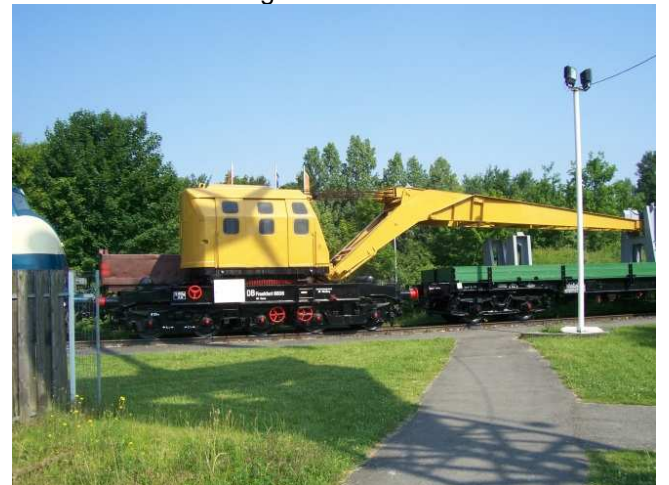
Track maintenance crane and boom car.
