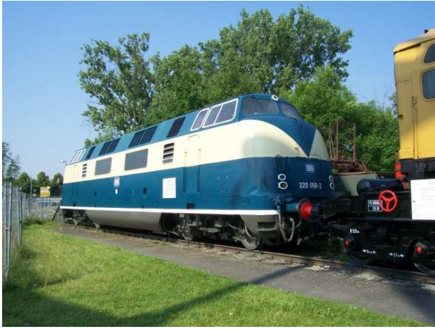
Modern double ended Deutsch Bundesbahn diesel locomotive.
