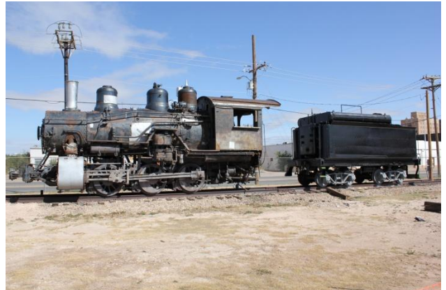
0-6-0 Switcher with lots of rust in front of the Clovis Depot
