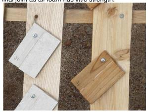
The second failure was the IC super glue (ACC) gel also on two pieces of metal. Both of these just fell apart. The MARINE GOOP is holding strong even on the metal pieces. Perhaps in the summer heat the expansion and contraction of the metal was too much for these glues. All the others seem strong as ever. Each piece has a one quarter inch tight overlap, was glued per instructions and clamped for 24 hours.
