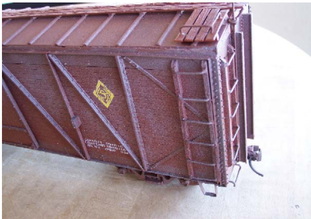
Side and corner of completed car. Note the corner steps visible in this view.
