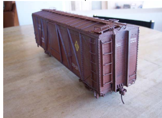
Overall view of the completed car. Note the 'crimped' metal roof, wood roof walk and corner platforms and the metal grab irons and supports for roof walk overhang.
