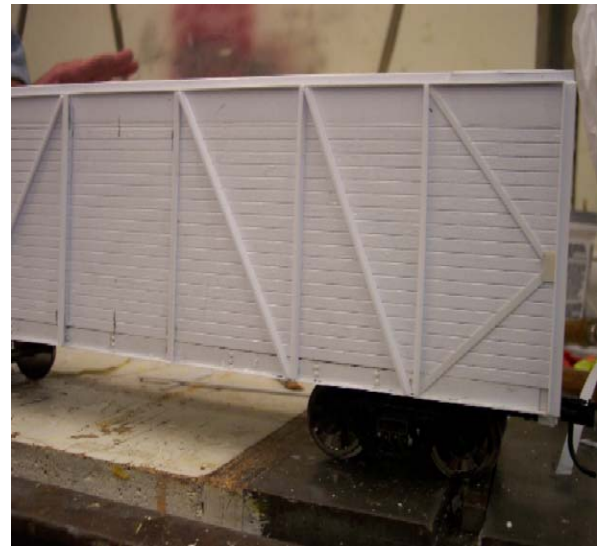
Here is the car with the vertical and diagonal bracing applied.
