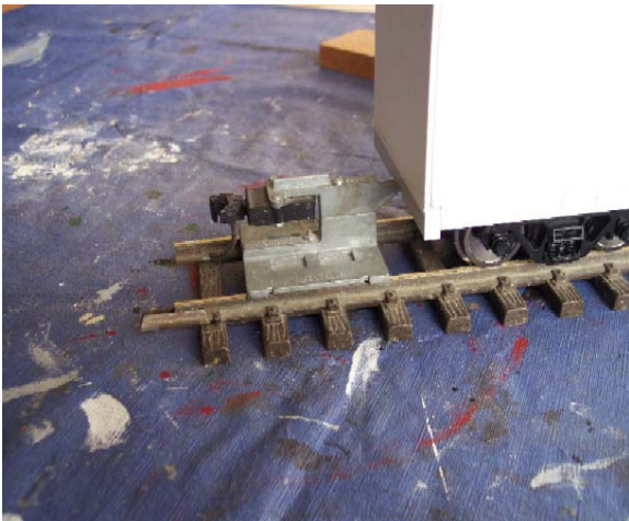
Coupler gauge slips into place after filing the end beam.
