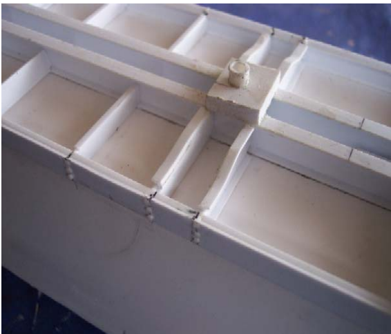
Kingpin and bearing block epoxied in place.
