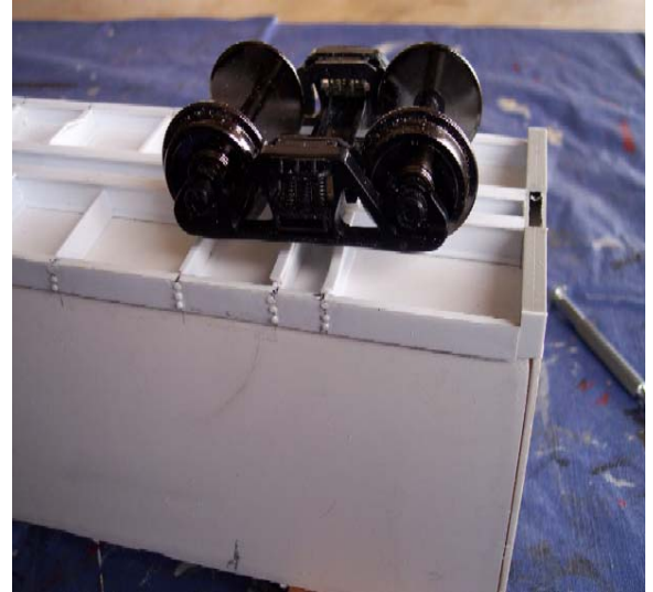
Kingpin shortened and truck in place.
