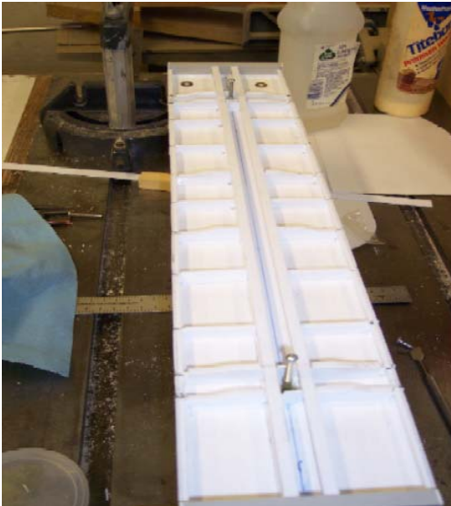
Nut being epoxied to car floor.
