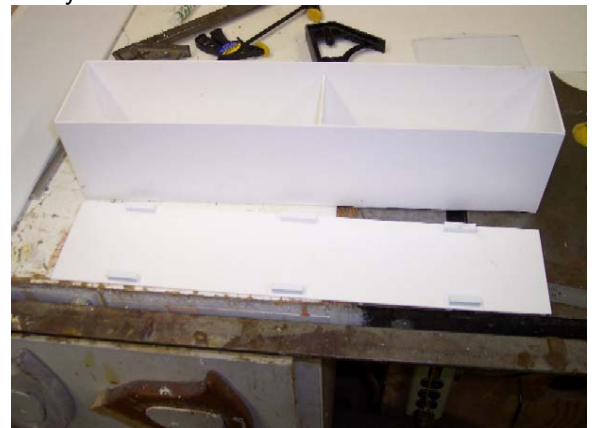
The hard to see center brace and roof brace block have been applied.
