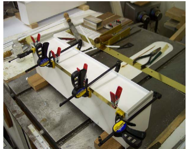
Gluing the side sill to the car.
