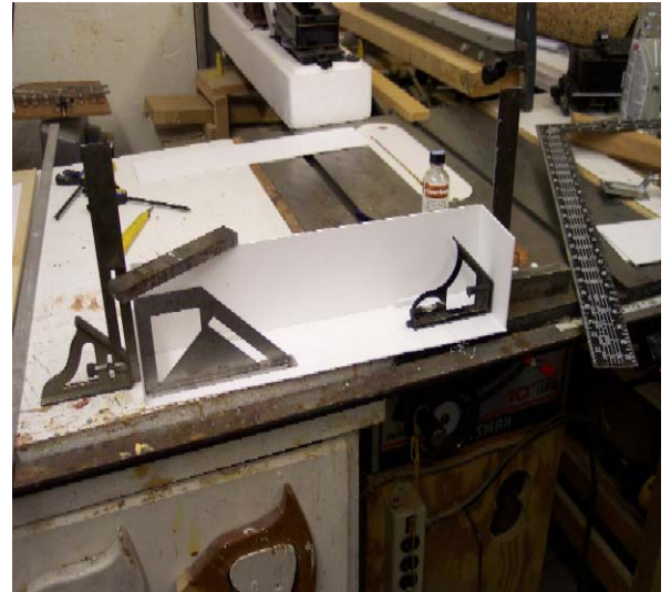
One side, the two ends and floor are glued with Plastruct's liquid cement.
