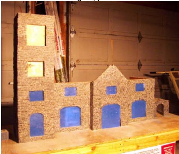
Plexiglas windows in place with the blue plastic protective wrap temporarily left in place.
