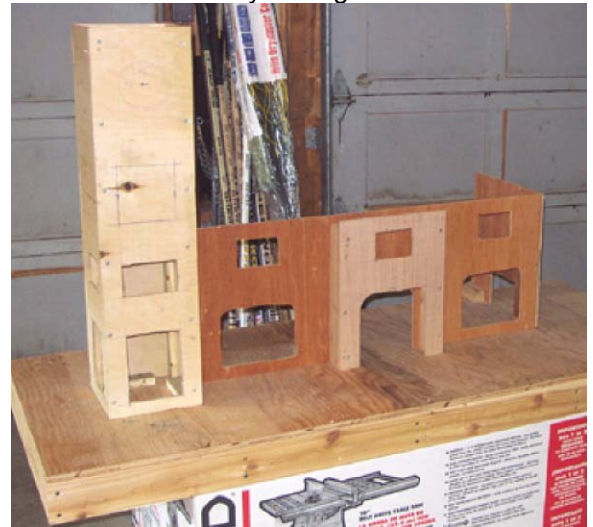
The plywood framing with roughly cut window and door openings.
