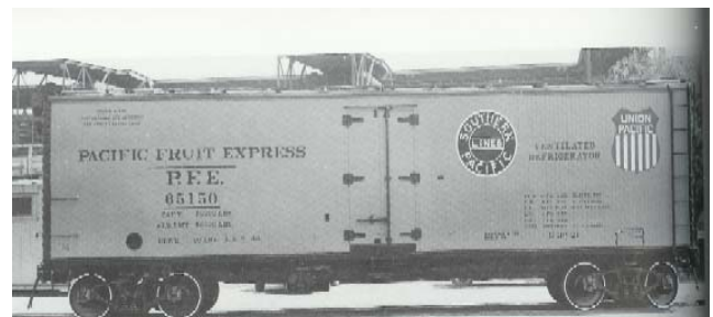
A Pacific Fruit Express wood car with metal ends and underframe
