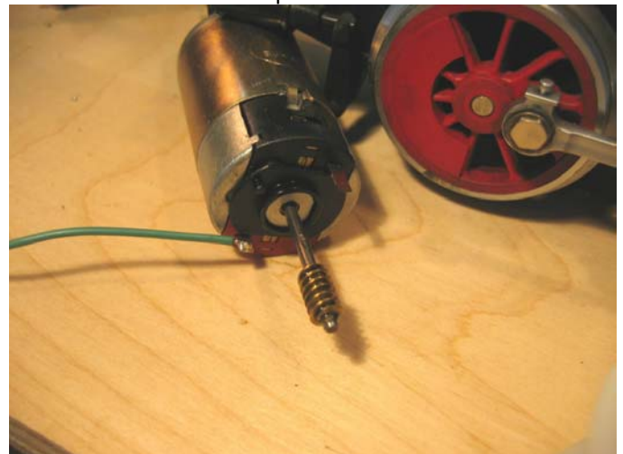
Figure 6 – New wire soldered to bent back motor tab
