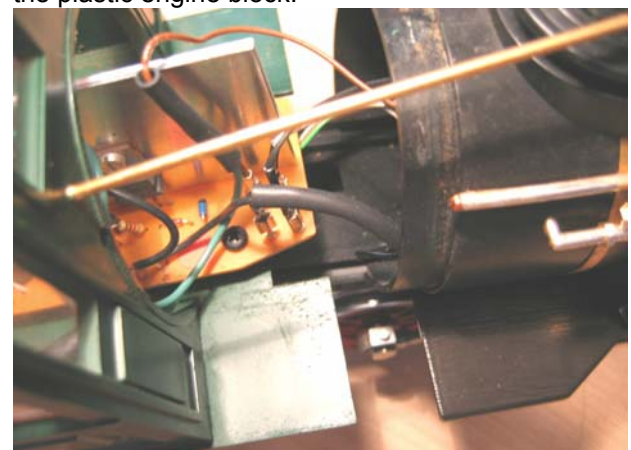
Figure 3 – Cab removed from boiler
