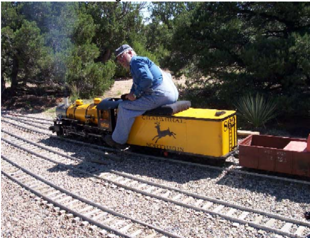
Shown here working up steam, Chaparral Northern railroad's coal fired 4-6-0 led our train.
