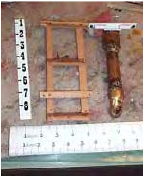
Spout crane (center), water level gauge, and water spout with hinge
