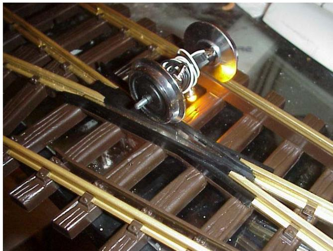
**Picture of wheels continuing to pick up current as they cross the new LGB large turnout frog.**
