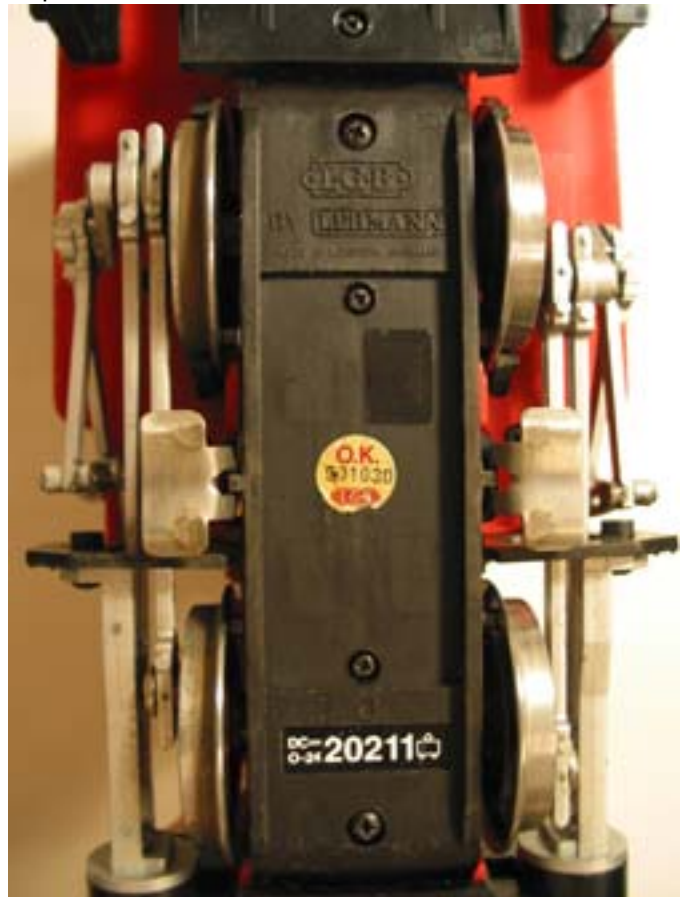
This bottom view of the LGB 20211 "Stainz" clearly shows the plastic traction tire fitted on the left rear wheel (upper left in photo). All other wheels are bare metal for conductivity of track power. (Mark Edwards photo)
