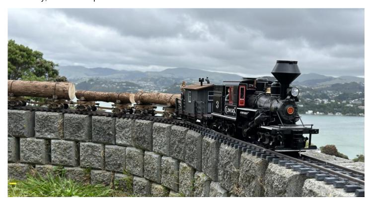
Rodney's Climax hauled logging train. Its battery powered, the battery in the support wagon behind - Photo John Robinson.
