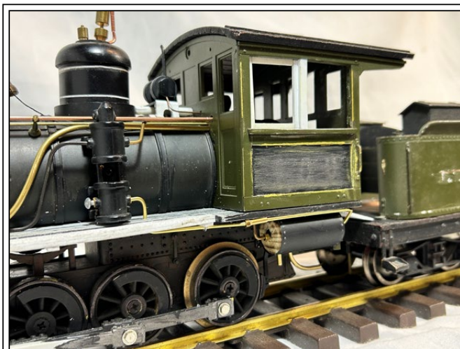
The air tank under the cab was made by wrapping a wood dowel with thin sheet styrene with rivets embossed along the edge. Brass and copper rod made new plumbing for air and water lines.
