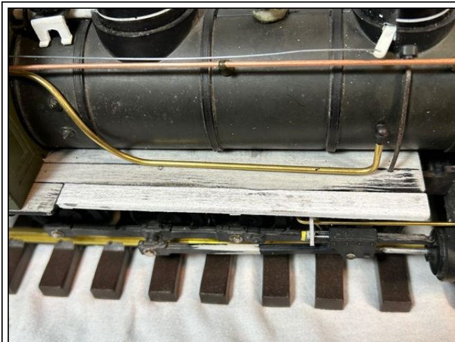
The author widened the running boards per the prototype. This was done simply by gluing additional styrene strip to the original running boards of the Aristo model.
