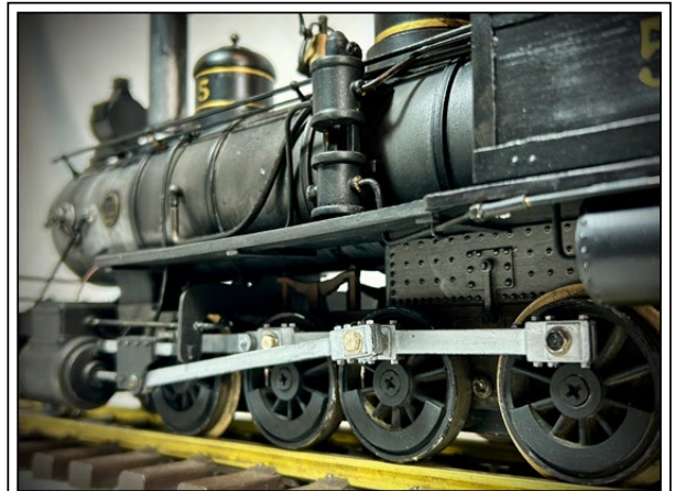
The author extended the main rod to reach the third set of drivers to match the prototype. The original model had the main rod going only to the second driver.
