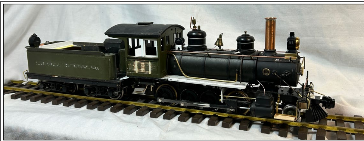
ET&WNC #5, rebuilt from #7 and #16, is ready for the paint shop.
