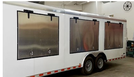
The modified automobile transport trailer with viewing windows closed.
