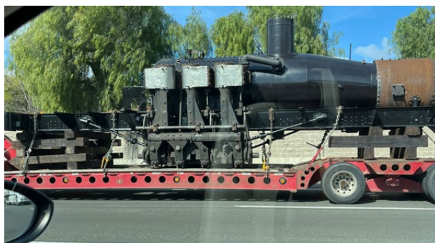
Rebuilt boiler for "Sonora No. 7" on road back home.
