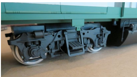
Finely detailed trucks and wheel set.
