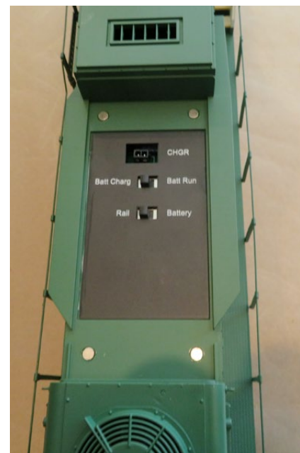
GP60 switches and charger plug under center fan assembly.
