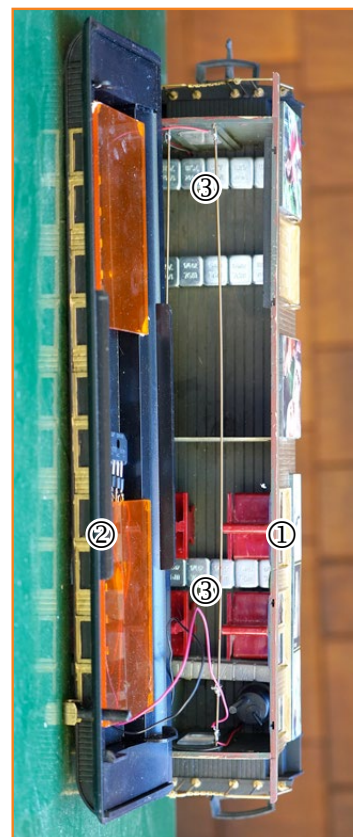
Interior view of a combine car shows ① the red seats and ② lighting set-up. ③ Weights were added over the wheels to keep the cars running smoothly.
