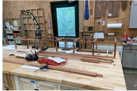
Engine shed post & beam frame in woodshop.
