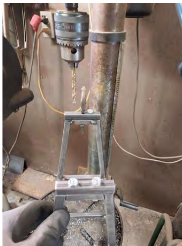
Photo 8 Top crossmember being attached with bolts.
