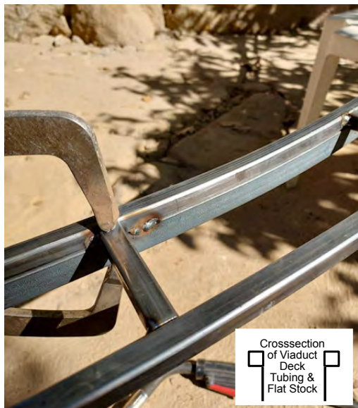
Photo 5 Attaching flat stock under the main rails to complete the bridge deck.
