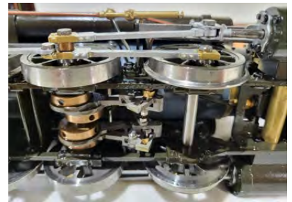
Efficient slide valve cylinders with a 1/2" bore drive a full working Stephenson valve gear.
