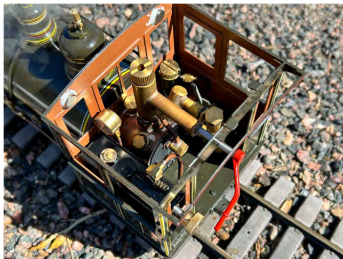
The cab fittings. The silver disks above the front windows are rare earth magnets used to hold the cab roof in place.
