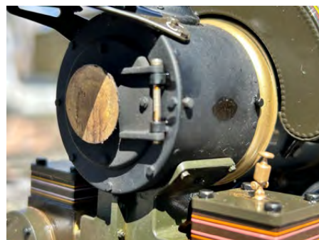
The adhesive used to hold the number plate and builder's plates to the firebox could not tolerate the heat and they fell off. Fortunately the smokebox was painted underneath the builder's plates so their loss isn't as noticeable as the missing number plate on the front.
