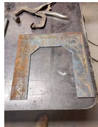
Photo 4 The cut-out backing plate.
