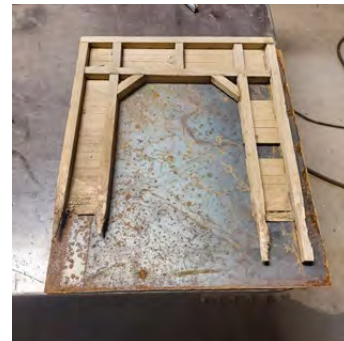
Photo 2 Transferring measurements onto the steel plate.
