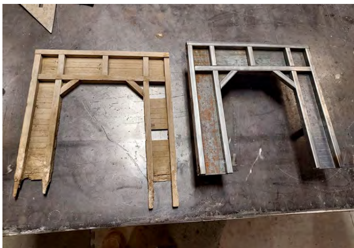
Old timber portal, New steel portal.
