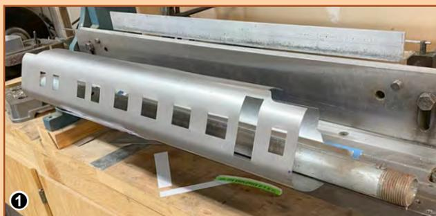
I drew up each car in a CAD file as a one-piece steel sheet metal part that had the windows and other profiles laser cut. The sheet was then rolled and bent over a steel pipe (photo 1) to form a complete tubular shell (photo 2).
