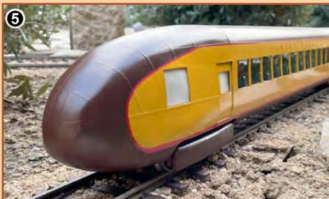
The front and rear of the train have complicated shapes, so I made those from basswood and finished with Bondo to make a smooth paintable surface (photos 4 & 5).
