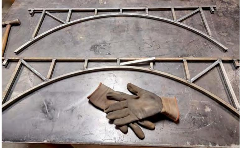
Photo 7 Fitting the cross braces.
