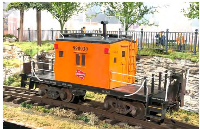
The finished model with light weathering and decals applied. The roof has a smoke stack (USAT), a small vent, roof walks (USAT) and distinctive railings. There's one problem. The truck-mounted couplers are hidden because of the length of the porches.
