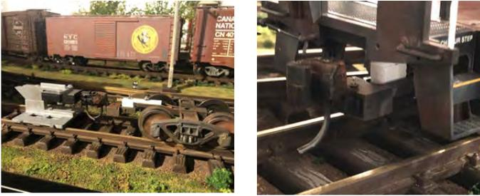
So, a bridge between the couplers and the bar from the truck had to be created. Here (in white) it is being tested to a Kadee height gauge. Prototype photos show the bar from the under-frame is heavy-duty steel and muscular.
