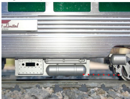
Stock. The bottom of the air tank is at the bottom of the brake assembly.
