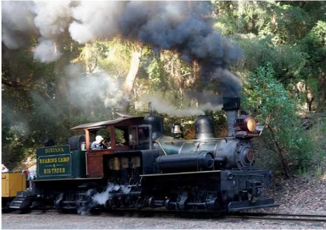
The Roaring Camp and Big Trees Railroad. In the middle of a grove, the two-truck Shay "Dixiana" backed up, gathered steam, and gave us all a dramatic run-by. She achieved speeds in excess of 16 mph. On the right, the Shay's hard-working cylinders, crankshaft and drive shafts.
