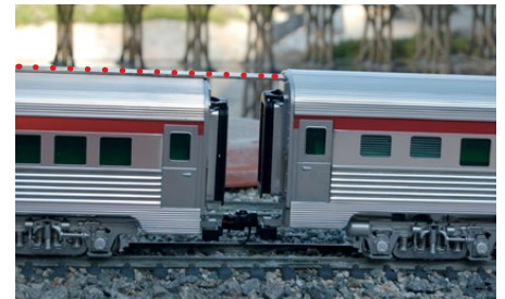
Modified coach (left) sits lower on its trucks for an overall reduction in height.
