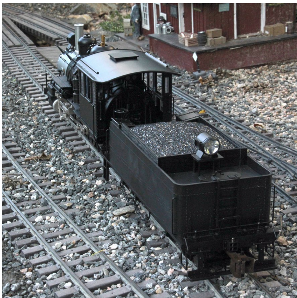
The Bachmann 4-6-0 seen from the rear. The coupler can easily be swapped out for a Kadee coupler, but legacy knuckle and hook-and-loop couplers are also included.
