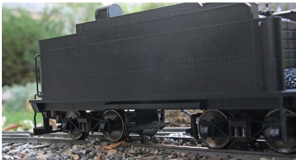
A poling pole (for moving cars on adjacent tracks) is cast into the engineer's side of the tender frame just above the wheels.
