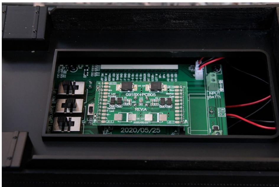
Under the removable coal load you'll find the "non-proprietary plug-and-play" socket, which can be used to easily install 3rd party control electronics. This is a "dummy plug" which enables the locomotive to run on traditional through-the-rail DC voltage.
