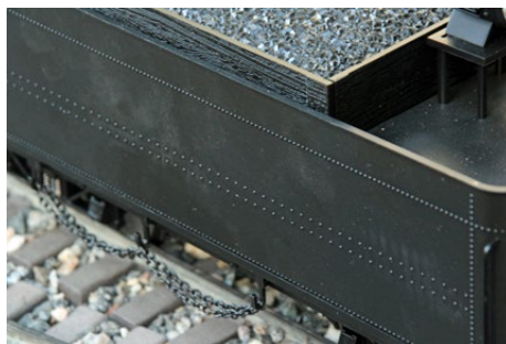
Scale rivets are the most noticeable difference on the tender, visually matching the details on the locomotive itself. Chains hang off the bottom of the tender frame.
