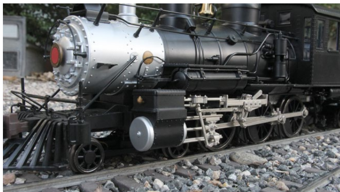
The detailed boiler and metal valve gear came from an earlier revision to this model. This version received a more prototypical, longer cowcatcher.
