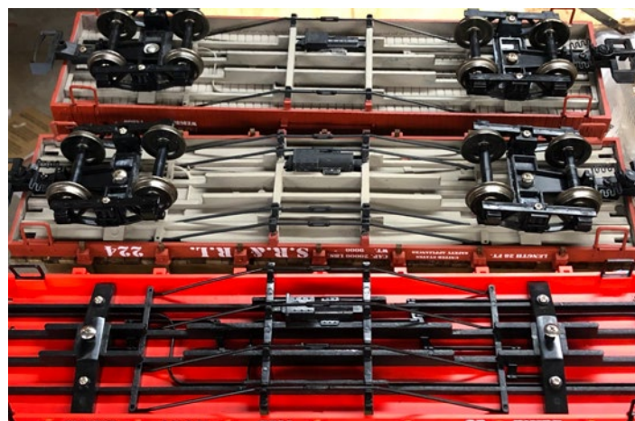
Bachmann freight chassis: original bottom, flat car with twin truss rods middle, and box car with single truss rods top.
